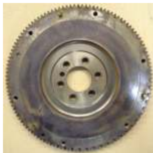
Fig 3: Flywheel friction side and back
