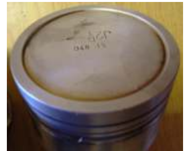
Fig 6: Permitted dished piston
