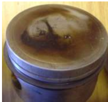
Fig 2: Permitted piston long skirt raised crown 0.75mm stamped 390 15
